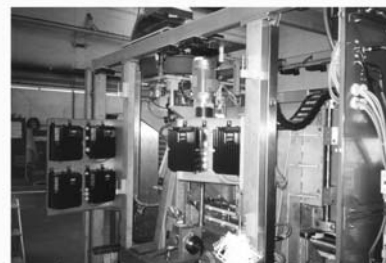
Illustration 1.13: Decentral motor controls integrated in packaging machine
